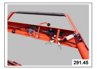
The second adjustment screw is under the drum screens on the frame
