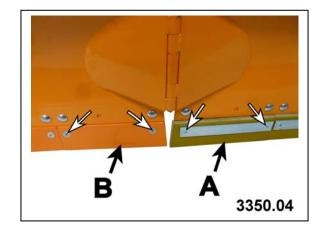
The interior scraping egdes are to be installed so that the incline is to the inside.
