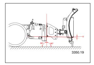
**P1** Standard position upon delivery This is the highest position of the adapter plate.
