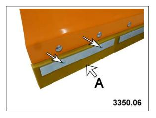
Secure steel scraping edges (B) in hole pattern.
