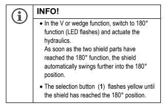
☑ Both LEDs (2 / 3) light up green as soon as the shield reaches the 180° position and is 90° to the direction of travel.
