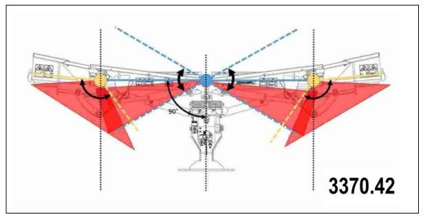
The outer shields can only be actuated if the corresponding inner shield is not in the collision zone. The buttons (3 / 4) light up blue.
