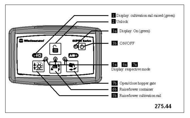
In principle, the controller must be activated for operation via button 3b "On/Off".
