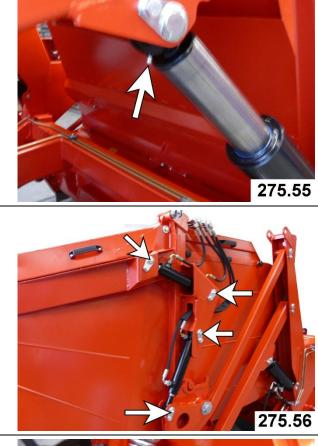
8.4.7. Pivoting axle Bearing bushing
