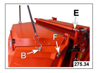
Bring the hopper gate into position for insertion.
