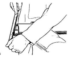
Smooth off division edges, remove chips carefully. Lubricate sliding profile.
