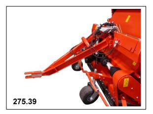
• fits the tractor if you change the tractor. Adjust the height of the drawbar if necessary.
