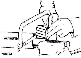
Cut off the inner and outer sheath tube evenly.
