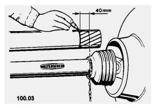
Cut off the inner and outer sliding profile by the same length as the sheath tube.
