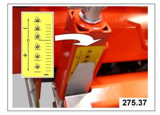
After the adjustment has been made using the handle (F), turn the adjustment spindle downwards to secure the adjustment in place.
