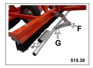
Tighten clamping screws (G).
