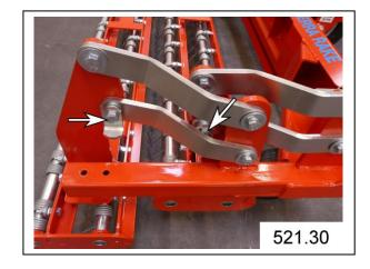
Secure the tension spring with long eye bolt (C) from the outside, instead of the removed screw on the right, with washer, spring circlip and screw (see figure 521.31).
