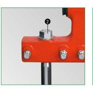
The integrated system for mounting and demounting tines allows the quick and trouble-free mounting of the conical 20 mm and 25 mm tines.
