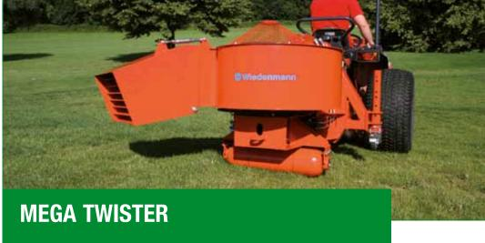
AttachmentstandaPT0 drive540, 1Air volume390 mExhaust velocity50 m/sSwivel angle230 °Power requirement30 kW
