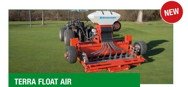
Working width approx. 160 cm and 1,500 holes/500 slits per m<sup>2</sup> Up to 3 cm work depth Rear attachment Cat. I or II, optionally with carriage Availability of brushes in various types of hardness Speed independent seed distribution from 1 g/m<sup>2</sup> to approx. 30 g/m<sup>2</sup> Approx. 1,100 kg lifting capacity
